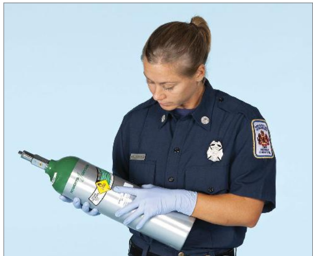
Figure 8-14 | Oxygen cylinders are marked with a yellow diamond that reads "Oxygen" and, in the United States, typically have green markings.
